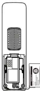
3. Slide the battery compartment cover towards the center of the handset until it clicks into place.
