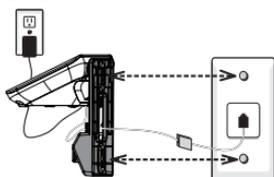
4. Align the holes on the bracket with the standard wall plate and slide the bracket down until it locks securely. Bundle the telephone line cord and power adapter cord neatly with twist ties.
